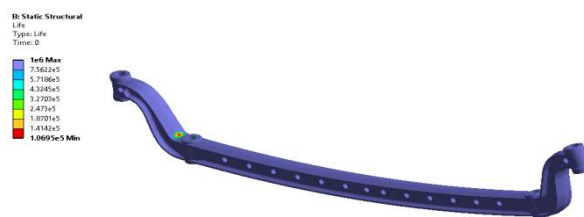
fig 7.0 Shows axle with holes fatigue life
