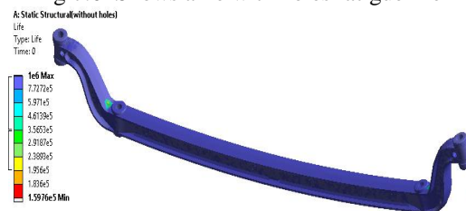
fig 7.0 Shows axle with holes fatigue life
