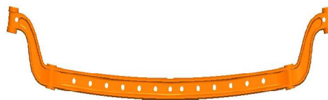
Fig 5.0 Dead Front Axle
