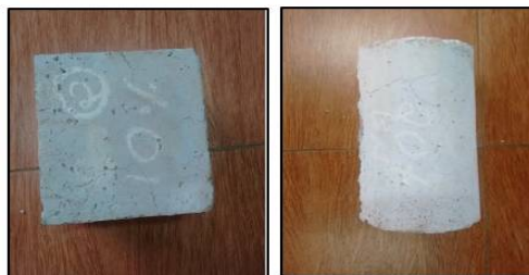
Fig. 5. Change in colour found in specimens subjected of 800°C
