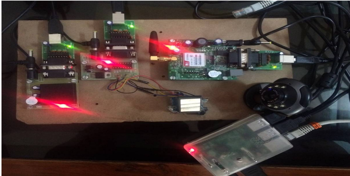
Figure 5: RFID reader, Fingerprint Scanner, Camera and GSM/GPRS Module is interfaced with embedded board
