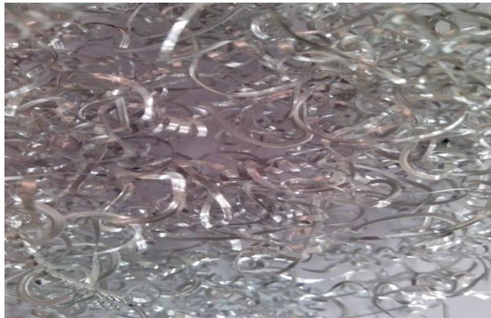
Fig -2: chips for pure aluminium.
