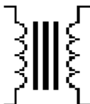
Figure: Transformer Symbol
