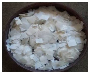
Fig.1. Square Pieces of Plastic Waste Admixture
