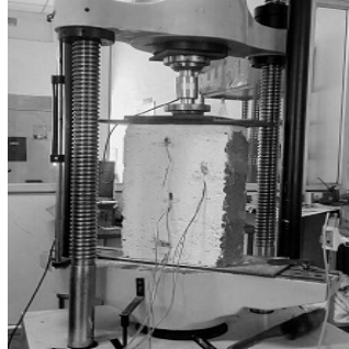
Fig.6 Compression testing of rammed earth prism
