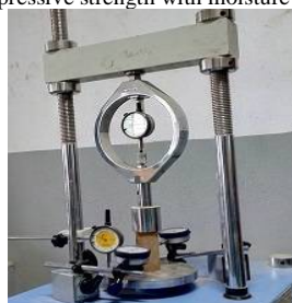
Fig.3 vertical and horizontal deflection measurement of ucc samples.
