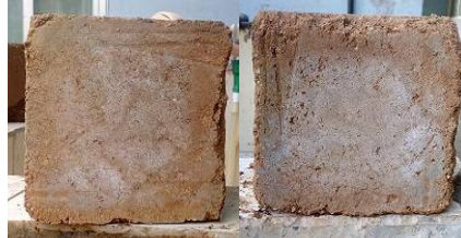
Fig. 9 Exposed face of the cube before and after the spray test
