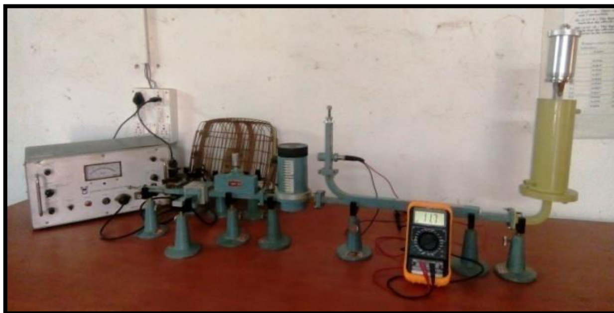
Figure 1. X-Band Microwave Technique Experimental Setup with Liquid Dielectric Cell.
