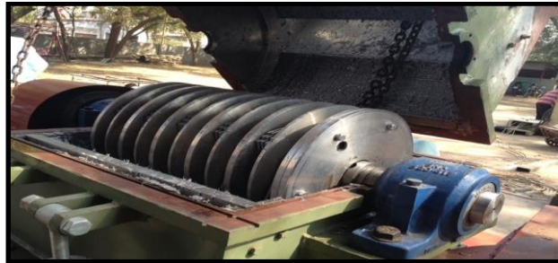
Fig:1 Rotor assembly of Hammer Mill
