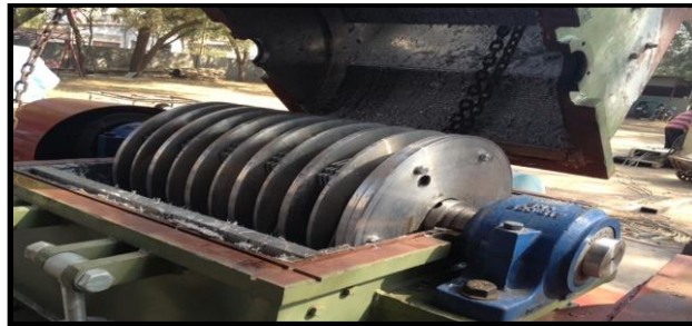
Fig:1 Rotor assembly of Hammer Mill
