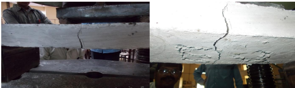
Fig. 13. Typical side view of crack pattern for 40mm and 50mm thick panel
