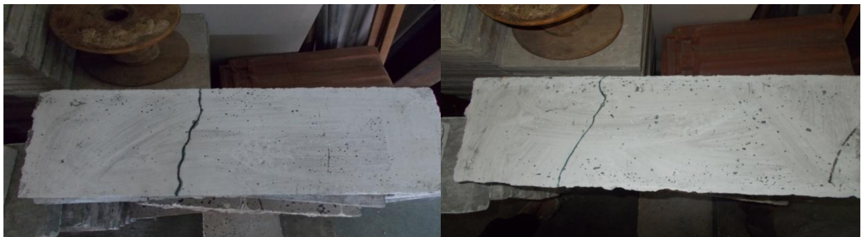
Fig. 11. Top view of crack pattern for 20mm and 30mm thick panel
