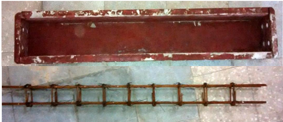
Fig. 1 : Reinforcement and FormWork Details of Specimen
