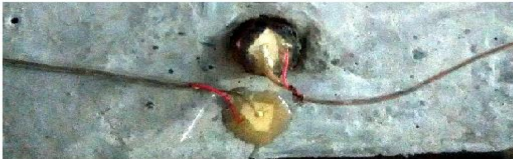
Fig 3: Surface Bonded PZT and Resuable PZT on Precast Beam
