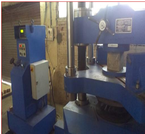
Fig 3. Testing of concrete cubes
