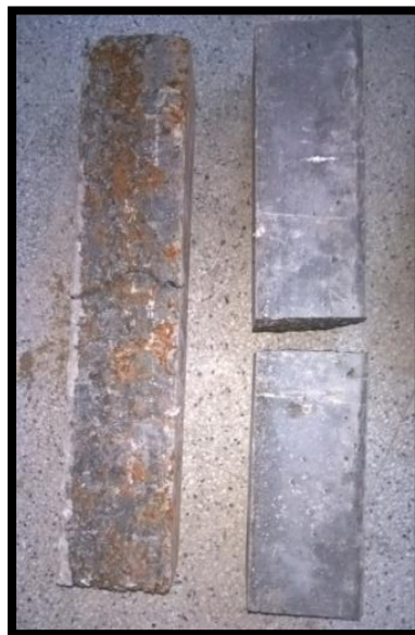
( ii)At Failure of beam specimen with fibres does not break and without fibres breaks.
