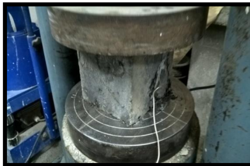
Fig.4. Failure of cube with breaking completely due to fibres
