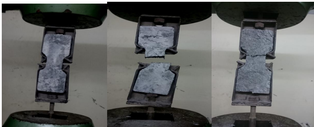
Fig.7. (i)Bracket Specimen(ii)Breaks at failure without fibre (iii) Does not break at failure with fibres.
