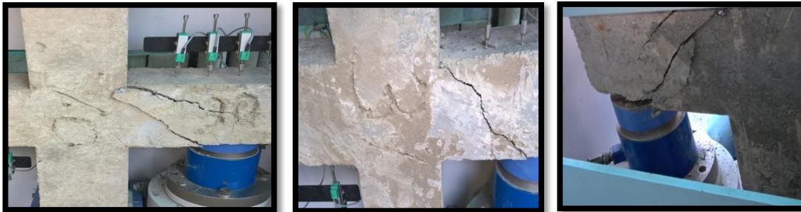
Fig.8 (i) RC Joint 0% Fibre Cracks (ii) RC Joint 3% Fibre Cracks (iii) RC Joint 0% Fibre Backside Cracks
