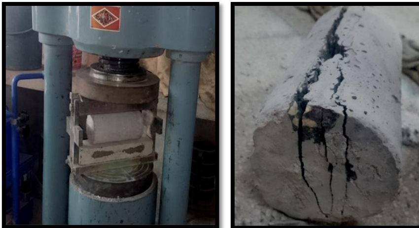
Fig.5. (i) Cylinder before test (ii) Cylinder at failure does not break due to fibres
