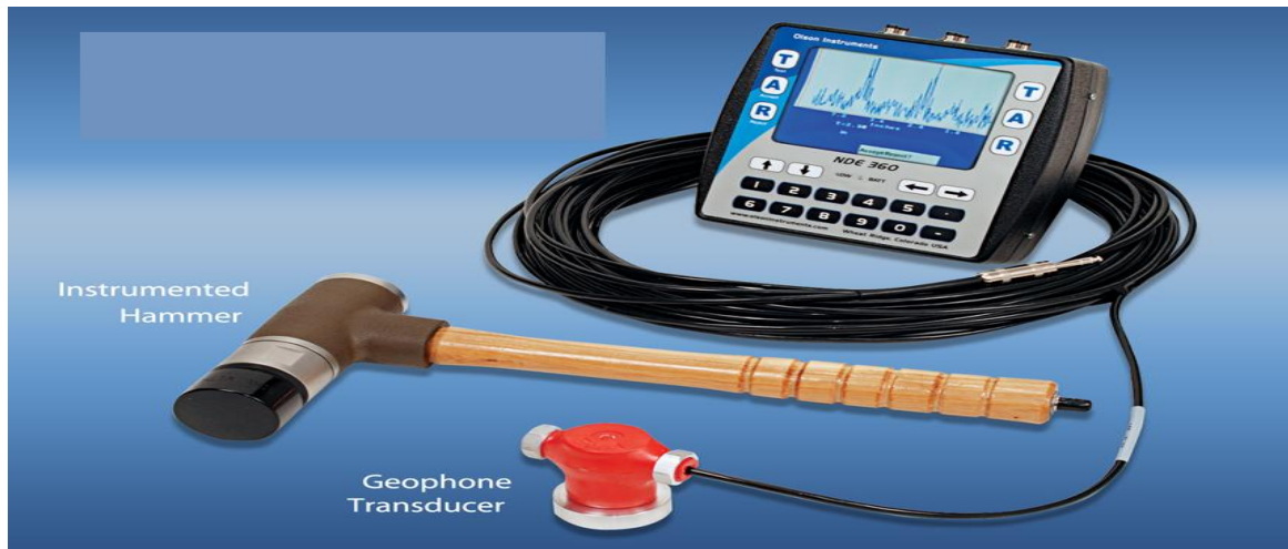
Fig 1: Slab Impulse Response Testing Apparatus
