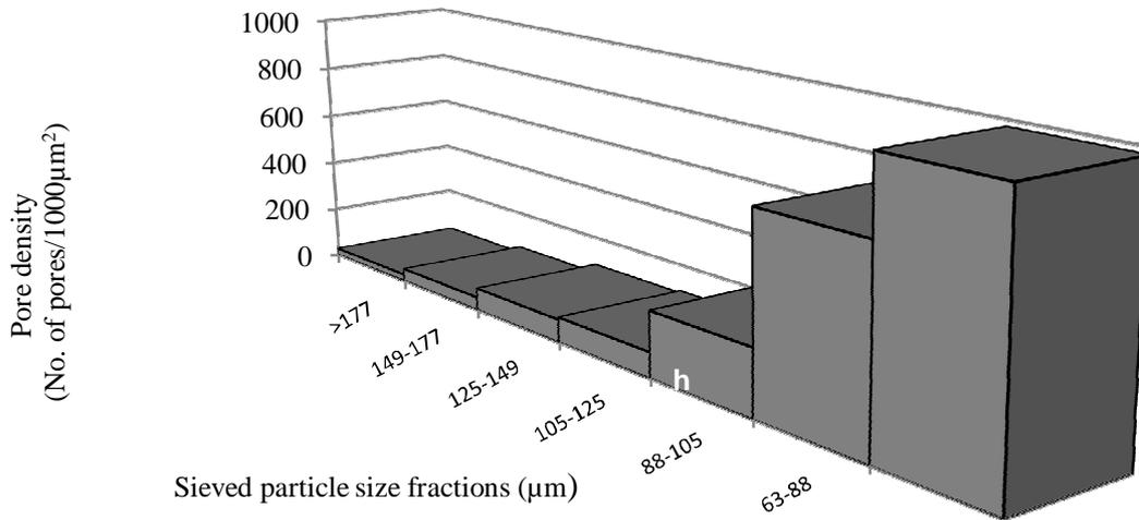
Figure 4. Pore density in particles of sieved particle size-fractions of carbon rich fly ash.
