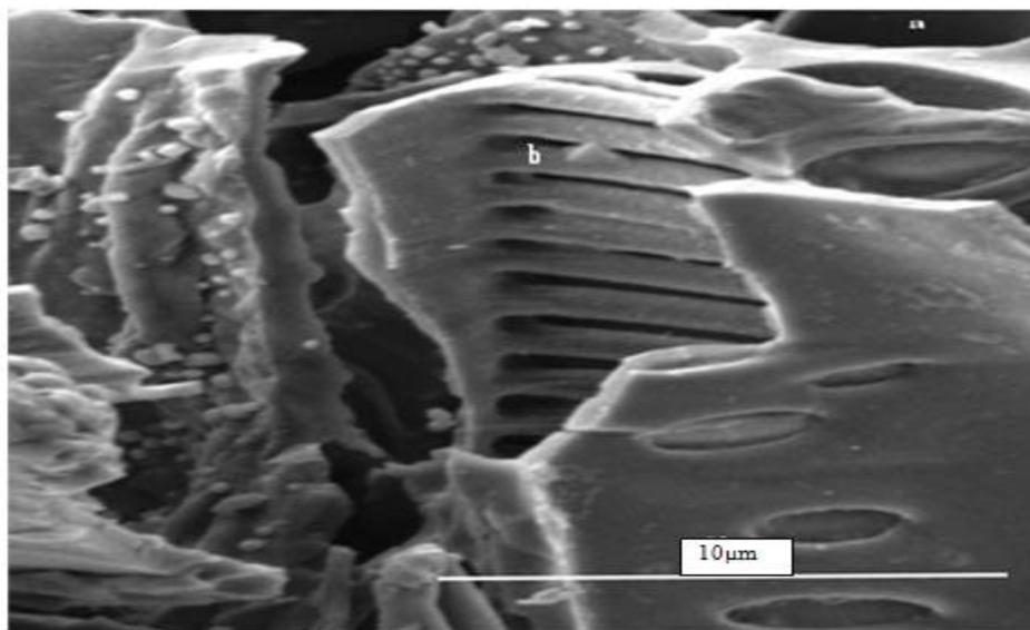
Figure 5. Porous structure of coconut shell-activated carbon; a) Pore vessel, b) Scalariform border pitting and c) Single border pit.
