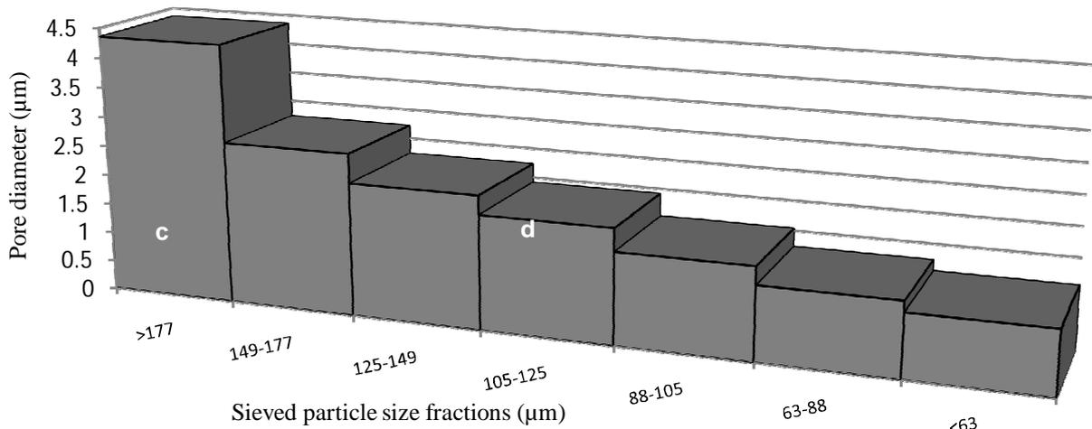
Figure 3. Pore diameter in particles of sieved particle size-fractions of carbon rich fly ash.
