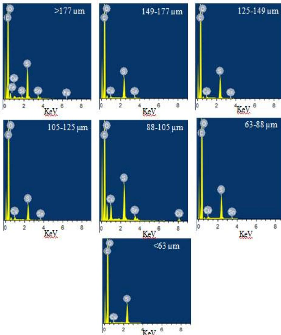
**Figure 1.** Qualitative and quantitative elemental analysis of sieved particle size fractions (SPSF) of carbon rich fly ash (CRFA) by energy dispersive X-ray spectroscopy (EDS)
