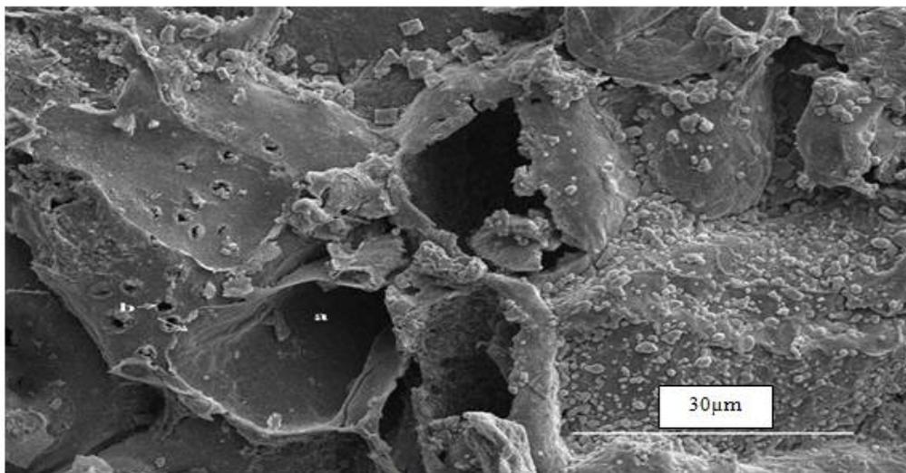
Figure 6. Porous structure of coconut shell-activated carbon: a) Natural pore vessel and b) A water steam activated-pore.
