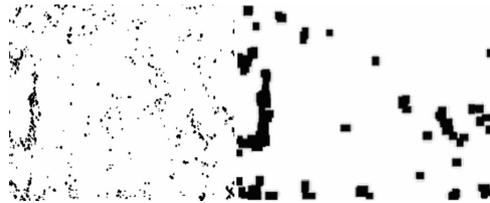
**Fig. 10** Results of the subtraction and dilation operations in order to segment the ledeburite.
