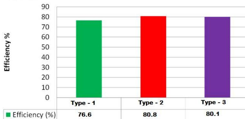
Fig 9 Volumetric Efficiency for different piston configurations
