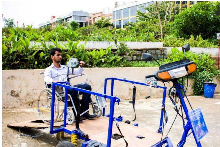
Fig. 3.1 User boarding the vehicle using the mechanical propulsion system
