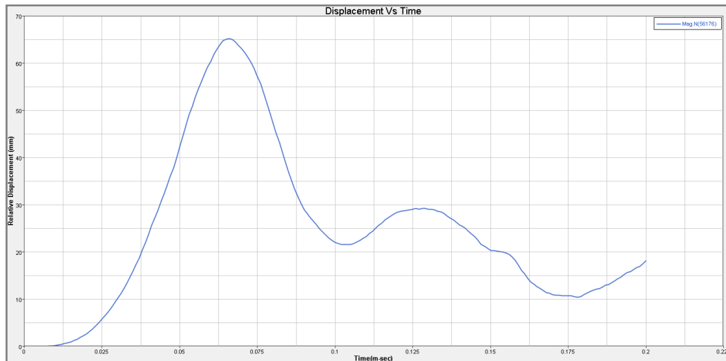
Fig.12: Displacement verses time plot in transverse direction.
