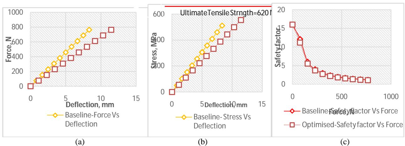
Fig.16.(a) Graph plot of Force vs.Deflection, (b) Plot of Stress vs.Deflection,(c)Graph plot of Safety factor vs. Force
