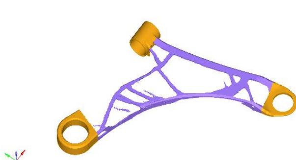
Fig.12. Element Density Plot
