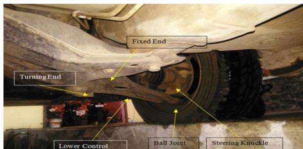
Fig.4. Connection of Lower Control Arm
