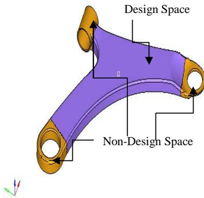
Fig.9. Optimized geometry
