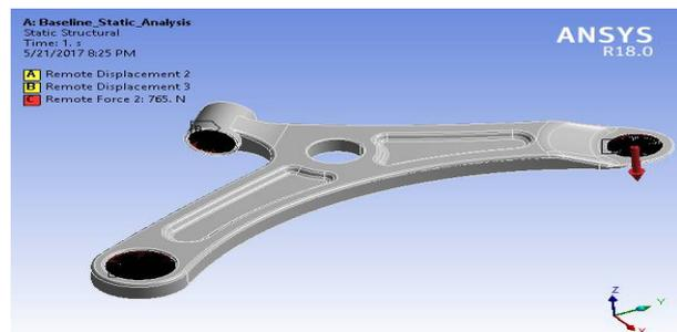
Fig. 5. Boundary Conditions of lower control arm.
