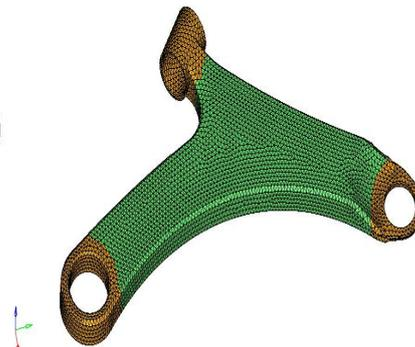
Fig.10. Mesh model for Optimization
