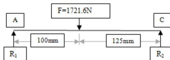
Fig.1. Line diagram for force distribution
