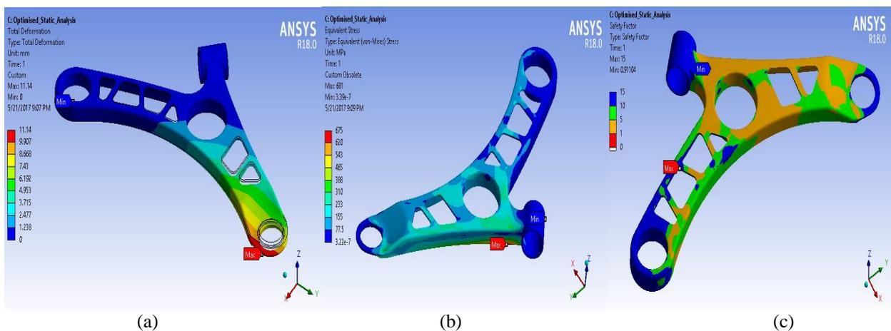
Fig.14. (a) Deformation Plot - Optimized design, (b) Max. von-Mises stress, (c) Safety factor for optimized design
