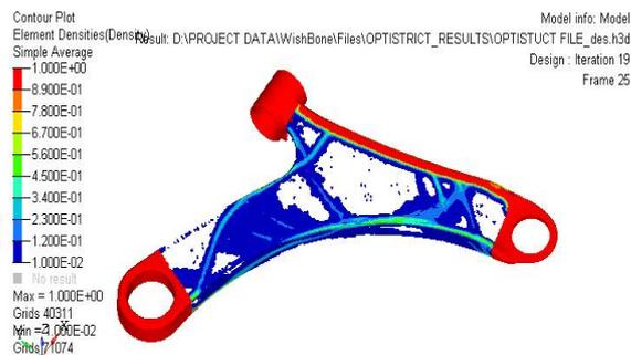
Fig.13. Element Density Contour Plot
