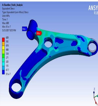
Fig.7. Equivalent Stress Plot
