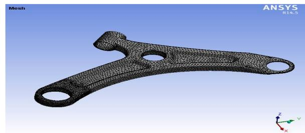
Fig. 3. Meshing of Lower Control Arm
