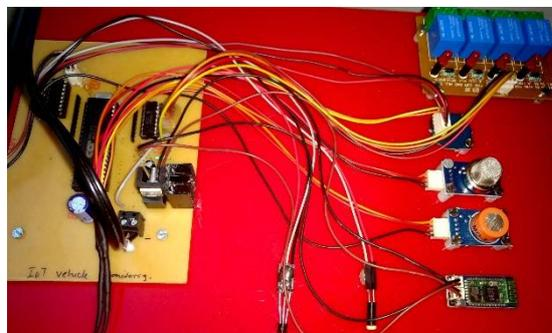
This figure displays the hardware unit of the system. It is installed in the vehicle. The system has a microcontroller, gas sensors, light sensor, accelerometer, temperature sensor, relay system and Bluetooth transmitter.
