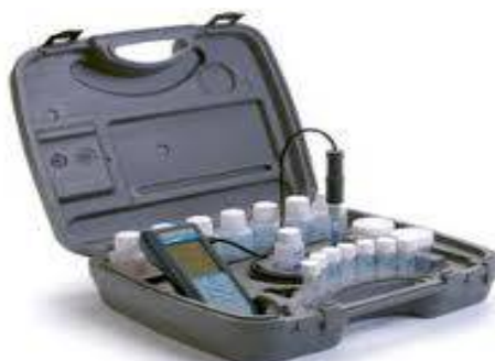
Figure 3.4 Portable Water Quality Kit (Merck)
