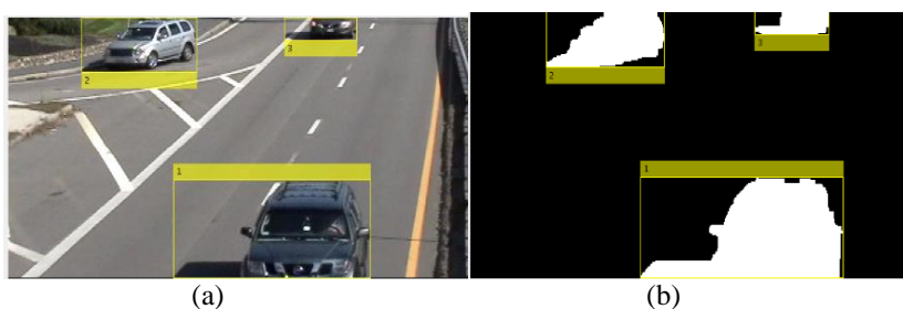
Fig. 5. Vehicle detection result from video (a) Actual frame (b) binary mask after morphological operation
