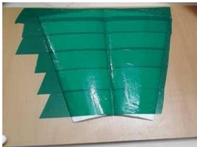
Figure 3: Initial Stage of Wing Fabrication
