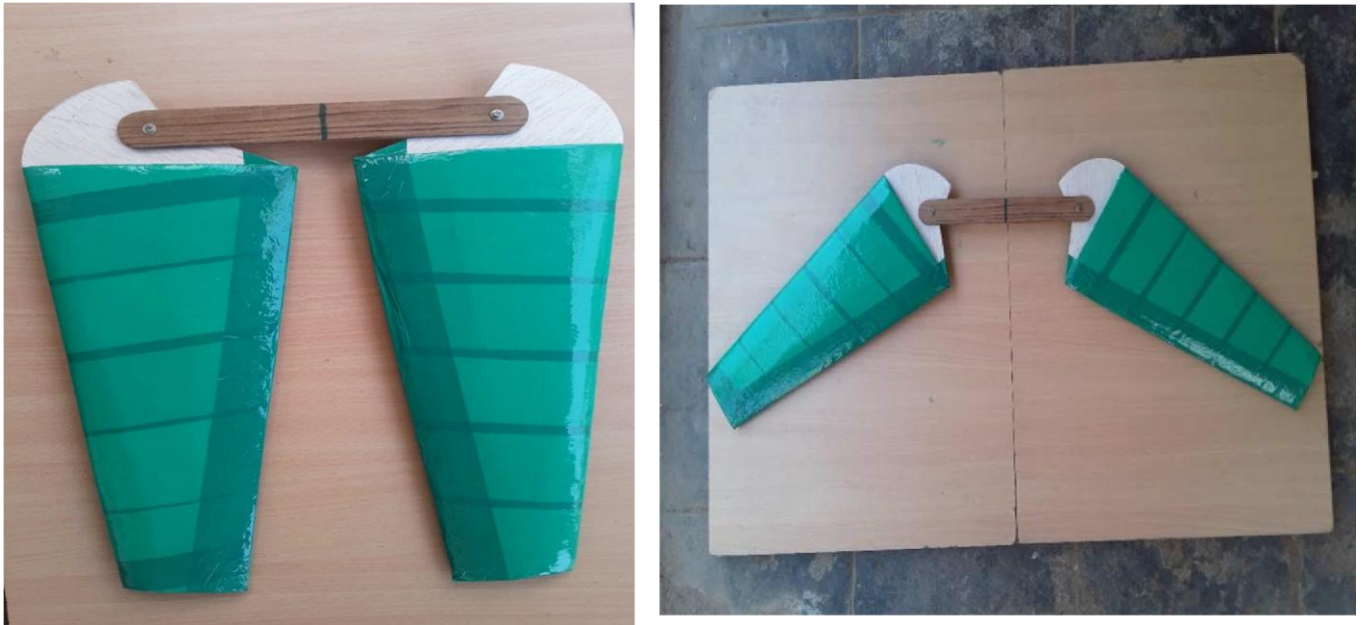
Figure 7: Wings ready to attach with fuselage section
