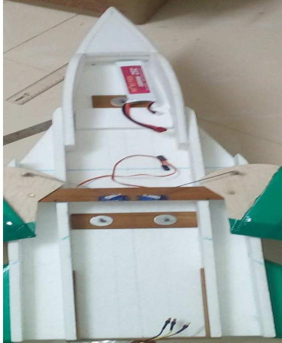
Figure 8: Wings attached with Fuselage and Nose section
