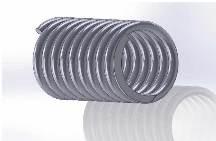
Fig.2 Three dimensional model of the valve spring
