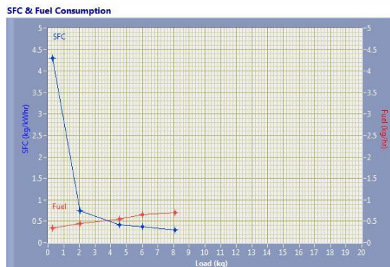
Fig 4.7 load vs (sfc & fuel consumption)
