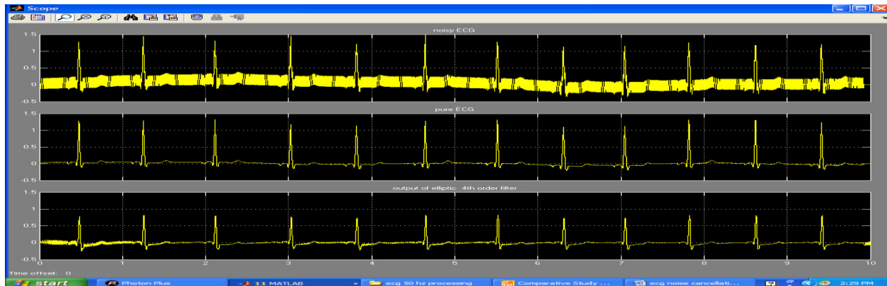
Figure 3.3: shows noisy ECG, pure ECG, output of 4th order elliptic filter
