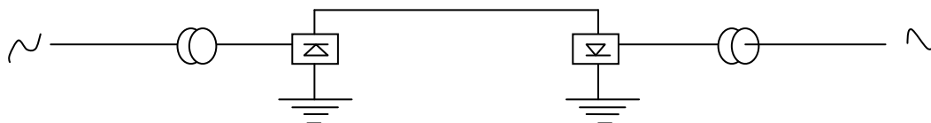
Fig1: Monopolar line with Earth Return
