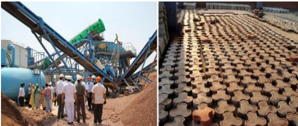
Figure.1 Delhi based first C & D waste plants of India, interlocking tiles made by waste material
