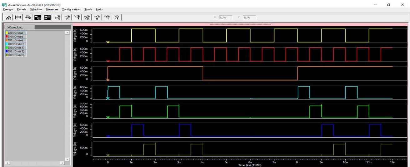
Fig. 6 Output waveform of CNTFET based 2:4 Decoder
