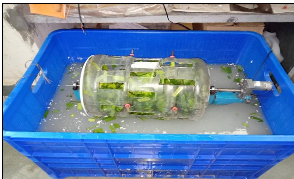
Figure2: Experimental Set –Up of RBC
