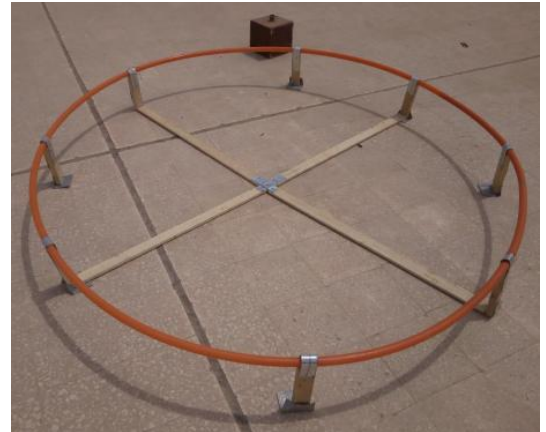
Fig.7, wooden pillars were stuck in the ends of the cross shape with PVC tubes
