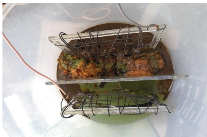
Figure2. Showing The Laboratory Level Leachate Treatment By Electrocoagulation Process.
