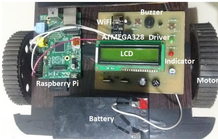
Fig5. Control system of vehicle overloading protection system.
