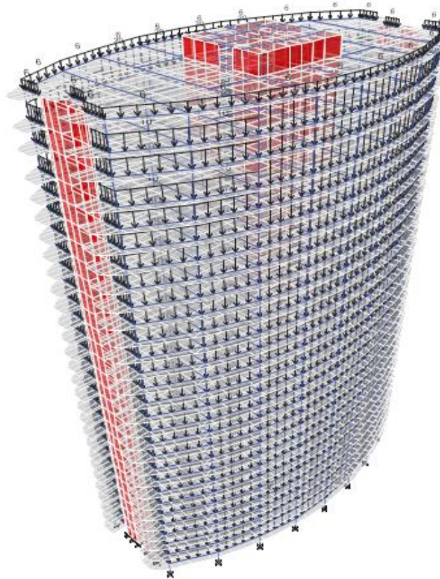
Fig 5: Wall load in 3D (Zone II & V)
