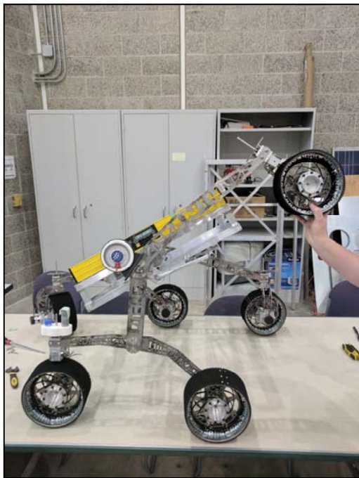
Figure 9: \beta = 60^\circ inclination of the left suspension rocker linkage. This was the most extreme inclination capable of PicusMartius without the bogie driving the rocker linkage past perpendicular with the ground.
