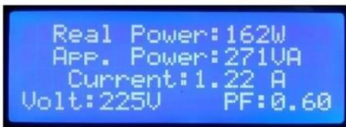
Fig4: Load condition before and after power factor correction
