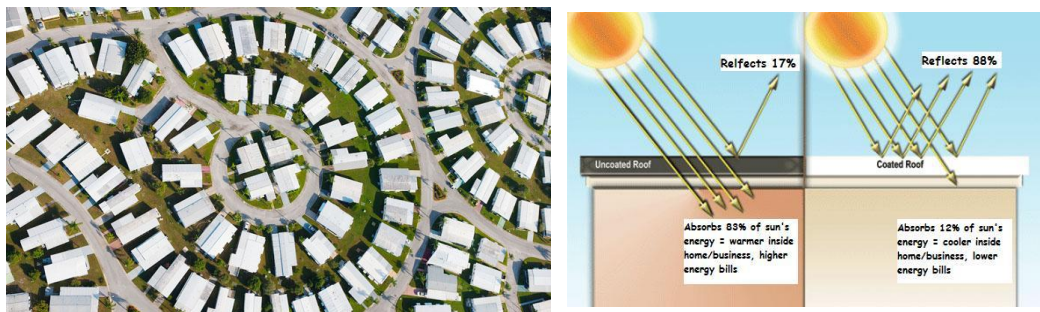
Figure 20: Translating cities roof line white – reducing heat gains Source http://www.gatewaygreen.org/white-roofs-a-new-sustainable-direction-for-cities/
