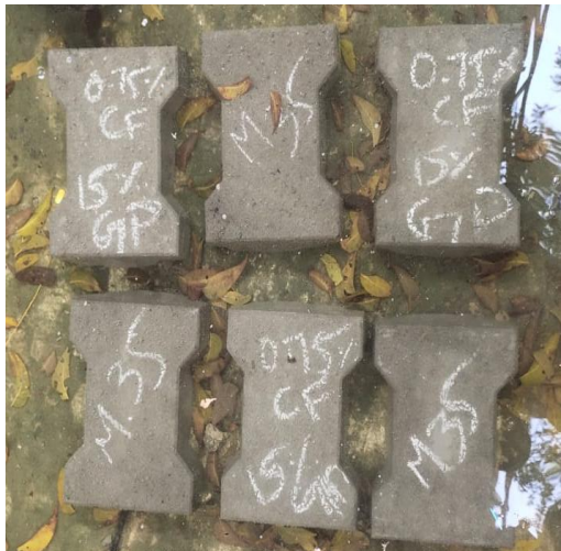
Fig.No(13) Curing of specimen
