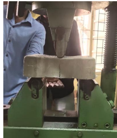
Fig.No(19)crack developed at specimen
