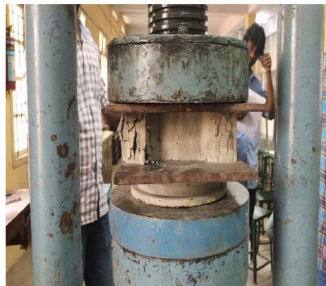
Fig.No(16) Crack developed at specimen
