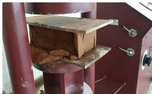
(c) Compressive strength test of blocks
