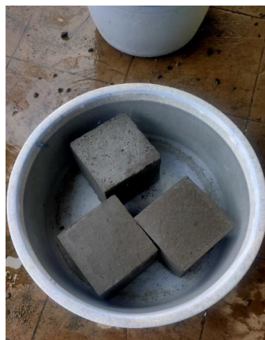
Image 3. Curing of concrete
