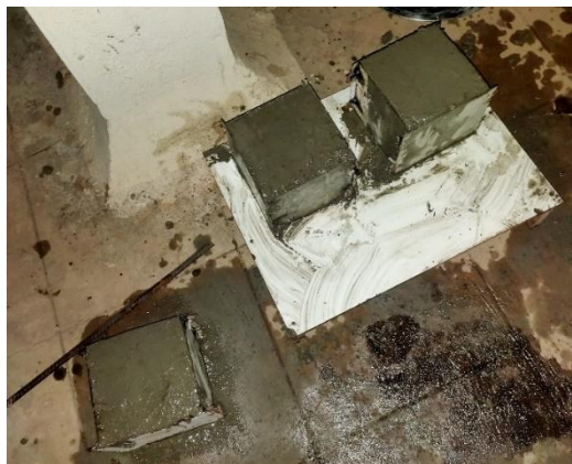
Image 2. Placing of concrete in still position for 24 hours
