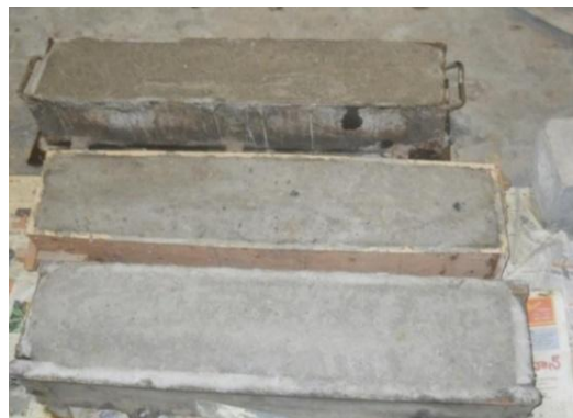
Image 5. Dried concrete beams
