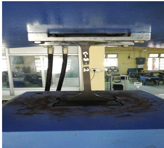
Figure 1.1 sample of coupon and dimension of the test specimen
