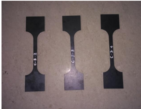
Figure 1.1 sample of coupon and dimension of the test specimen
