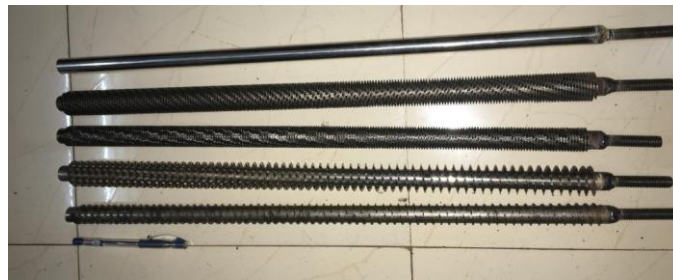
Fig.4. Plain and Spiral Fines Tube With Different Fin Geometry.
