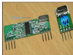
Figure No.2: RF Transmitter Module
