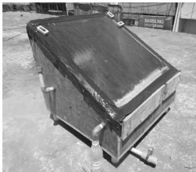
Fig7 Single basin double slope
