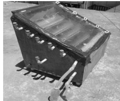
Fig. 8 Double basin double slope
