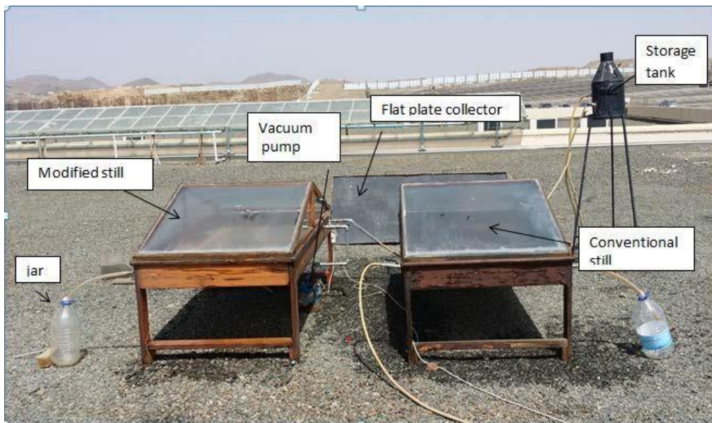
Fig.9 (a) Schematic Diagram of Experimental (b) Photograph of Experimental Setup.
