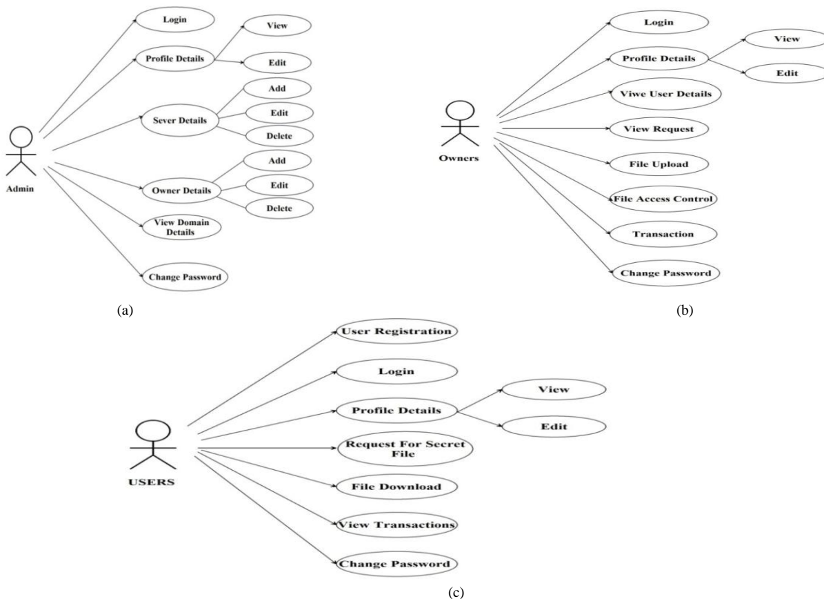
Fig 7. Use case diagram for Admin (a), Use case diagram for Owners (b), Use case diagram for Users (c).
