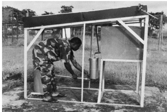
Figure9: Active carbon/methanol adsorption cooling system.
