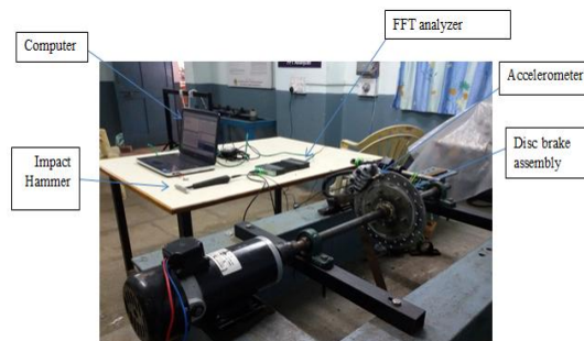
Fig.2 Experimental modal analysis set-up
