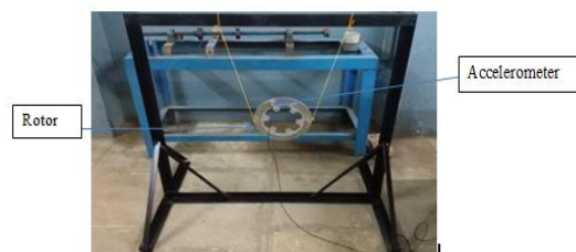
Fig. 3 Experimental modal analysis of Rotor
