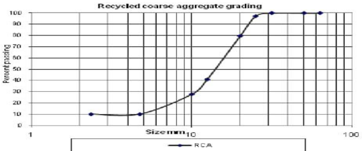
Graph 3: Particle Size Distribution Curve of Coarse Aggregate
