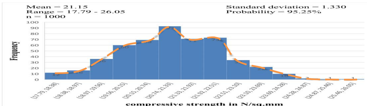
Histogram 4.7 showing Probabilistic Compressive Strength of 40% RAC
